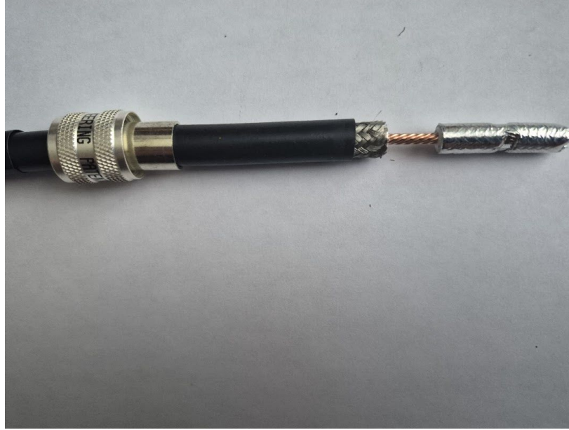
Remove Center Conductor Insulation. This May require some effort.
