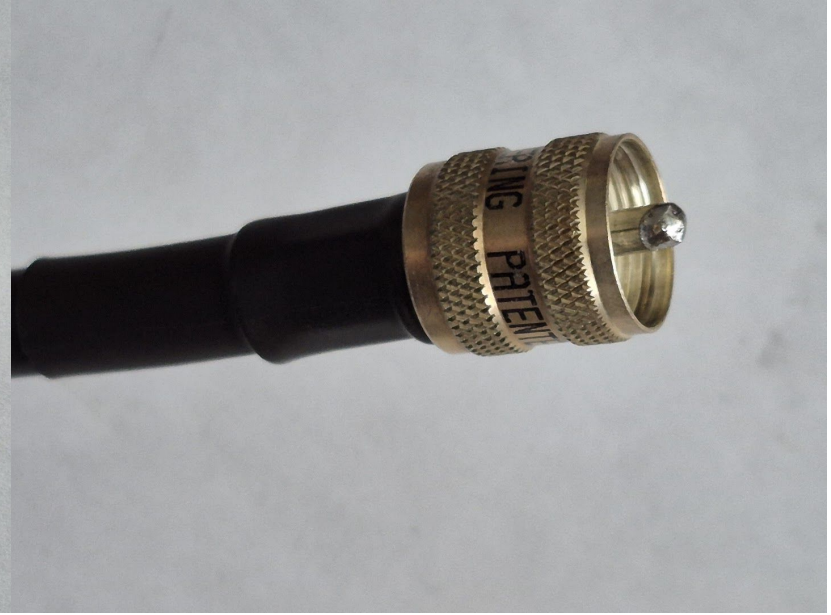
Solder Center Pin. Be careful not to cover pin with too much solder.
