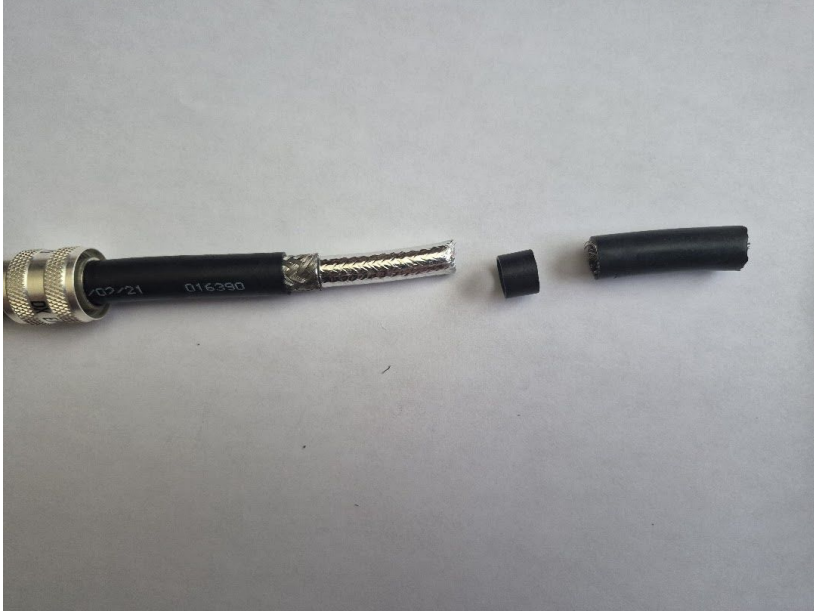
Remove Outer Insulation/ Braid
